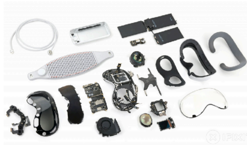
Cameras, LiDAR Scanner, Ambient Light Sensor, etc. on mixed reality headset (Apple Vision Pro as shown in the picture)
